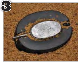
3 Carefully position the Method Feeder in centre of the mould and press firmly.
